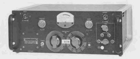
The Type 1133-A Frequency Converter is designed for use with the GR Type 1130-A Digital Time and Frequency Meter and the Type 1153-A Digital Frequency Meter. It can, however, be operated with other 10-Mc counters or as a general-purpose frequency converter with other accessory equipment.
